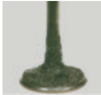
Intake valve before PI treatment.
