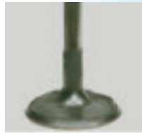
Intake valve after PI treatment.
