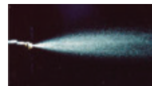
Injector spray pattern after PI treatment.
