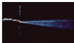
Injector spray pattern before PI treatment.
