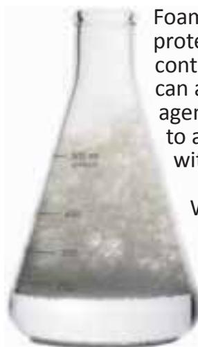
Foam in an oil system can lead to poor component protection and mechanical damage. Oil viscosity, contaminants, changes in surface tension and additives can all act as catalysts to the formation of foam. Anti-foam agents can stop foaming but require effective formulation to avoid **entrainment**—the entrapment of tiny bubbles within a fluid.
