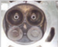
Combustion chamber before P.i. treatment
