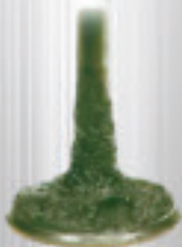
Intake valve before P.i. treatment
