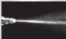
Injector spray pattern before P.i. treatment
