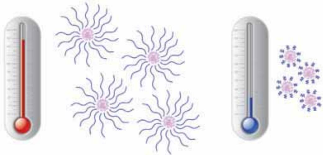
Figure 1.10 In warm temperatures (left), viscosity modifier polymers expand, raising the viscosity of the oil. When temperatures are cooler (right), viscosity modifier polymers contract, imparting no viscosity effect on the fluid.
