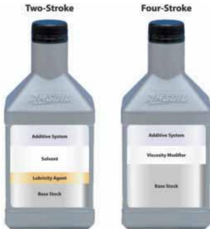
Figure 1.14 The emphasis of two-stroke oils, left, is miscibility with fuel (solvent) and reduction of friction (lubricity agent). The emphasis of four-stroke engine oils, right, is robustness because the oil stays in the system for an extended period of time.
