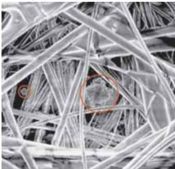
Figure 3.4 The interception filtration mechanism
