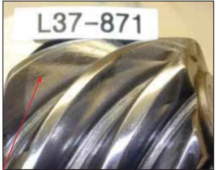
Pinion gear - original machine marks still present.
