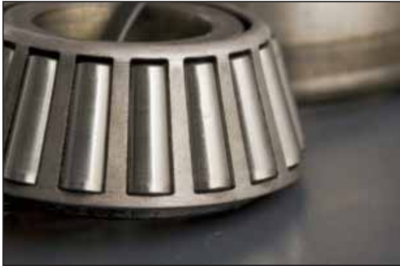
Pinion tapered roller bearing in like-new condition.
